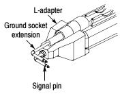
**L-adapter.** This adapter enables you to probe and ground at right angles to the device under test (DUT), while holding the probe parallel to the DUT. A ground socket extension that you insert into the ground socket of the probe is included.
