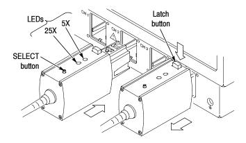
Figure 2: Connecting and disconnecting the probe
