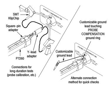
Figure 3: Probe functional check connections
