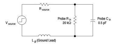
Figure 6: Ground lead equivalent circuit
