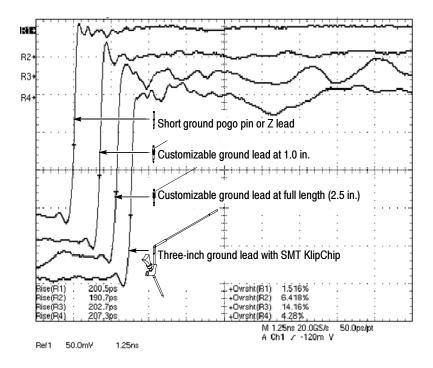
Figure 5: Waveform distortion from ground lead length
