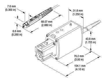
Figure 11: Probe head and compensation box dimensions
