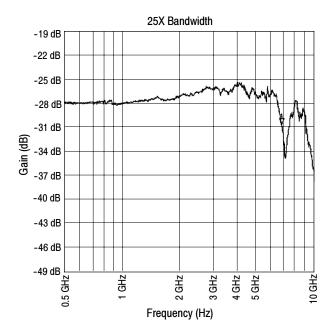
Figure 10: Typical bandwidth at 25X attenuation
