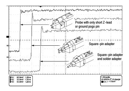
Figure 7: Typical effects of using the probe tip adapters
