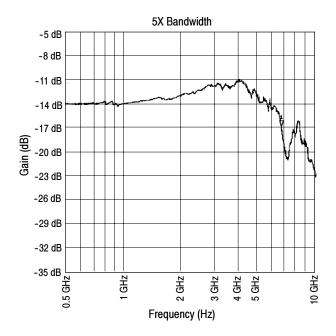
Figure 9: Typical bandwidth at 5X attenuation
