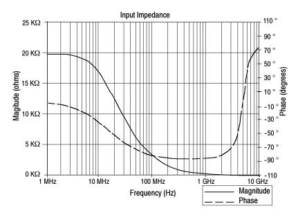
Figure 8: Typical input impedance and phase versus frequency
